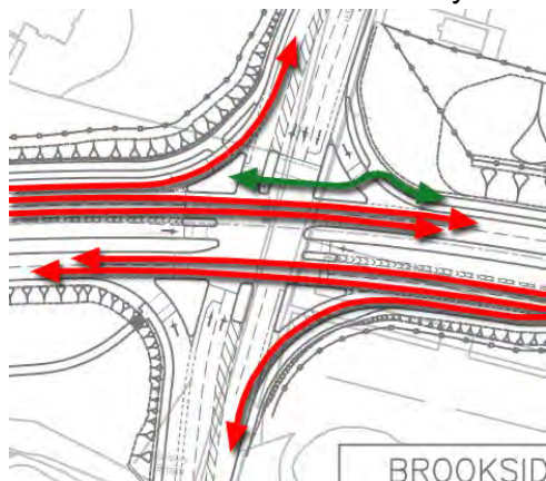
Diagram 6. One signal stage at Macclesfield Road
